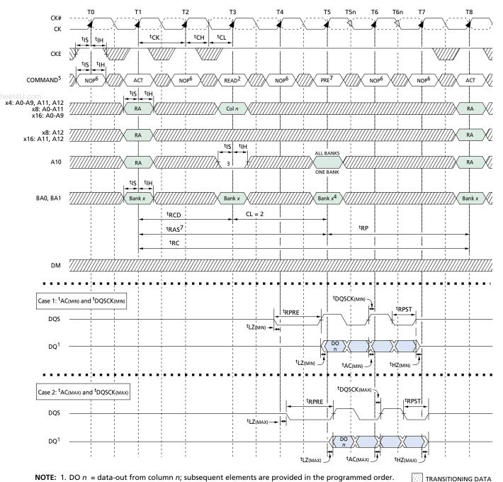
**NOTE:** 1. DO n = data-out from column n; subsequent elements are provided in the programmed order.
