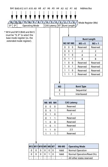
Figure 1 **Mode Register Definition**
