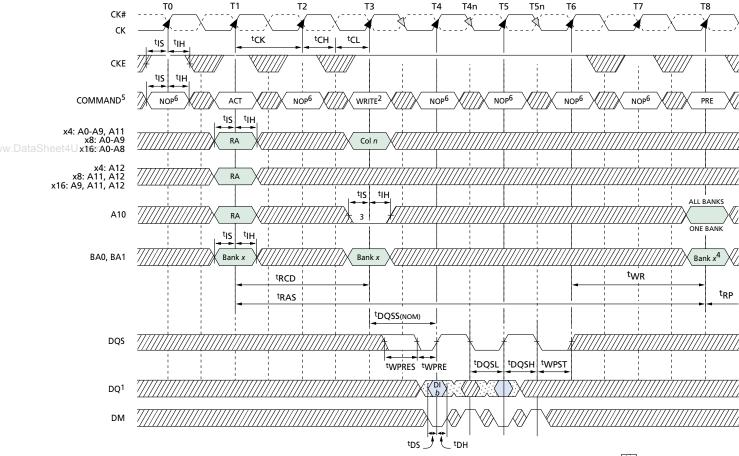
**NOTE:** 1. DI n = data-out from column n; subsequent elements are provided in the programmed order.
