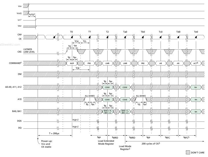
NOTE: 1. Vtt is not applied directly to the device; however, tVTD should be greater than or equal to zero to avoid device latch-up. VddQ, VddQ, Vtt and VREF must be equal to or less than Vdd + 0.3V. Alternatively, Vtt may be 1.35V maximum during power up, even if Vdd/VddQ are 0 volts, provided a minimum of 42 ohms of series resistance is used between the Vtt supply and the input pin.
