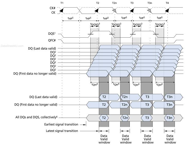
**NOTE:** 1. DQs transitioning after DQS transition define <sup>†</sup>DQSQ window. DQS transitions at T2 and at T2n are an "early DQS," at T3 is a "nominal DQS," and at T3n is a "late DQS"
