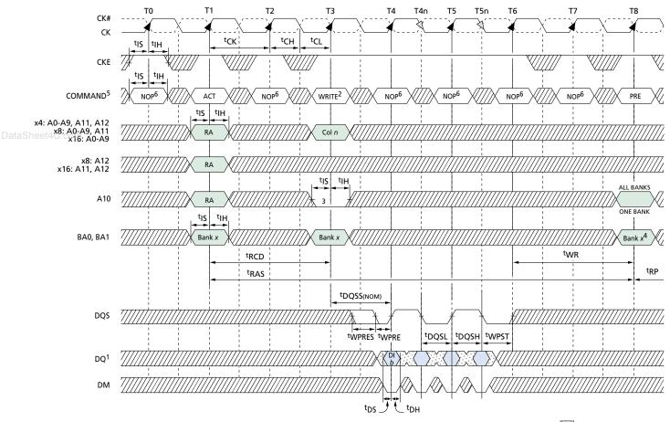
**NOTE:** 1. DI n = data-out from column n; subsequent elements are provided in the programmed order.
