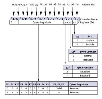
NOTE: 1. E14 and E13 (BA0 and BA1) must be "1, 0" to select the Extended Mode Register (vs. the base Mode Register).
