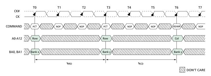
Figure 5 Example: Meeting  ${}^tRCD$  ( ${}^tRRD$ ) MIN When 2 <  ${}^tRCD$  ( ${}^tRRD$ ) MIN/ ${}^tCK \le 3$
